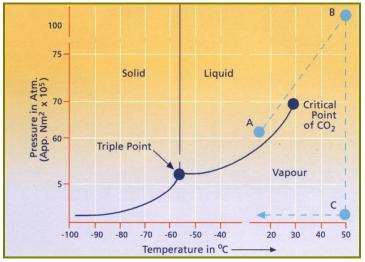
Figure 6.1 - Phase Diagram
