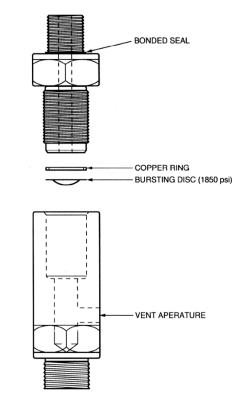
Figure 7.3: Safety Valve Assembly
